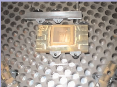
Close-up view of the die area showing fiber optic sensor, die and guide wires.
