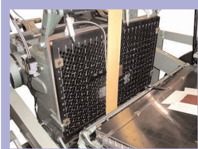
Hologram registration Unit set up on etched toggle base. Shows fiber optic sensor, wire guides, die and foil to the center of the toggle base.
