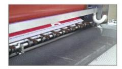
Thin Substrate Removal Kit prevents wrap-up of prints, resulting in a more reliable production line.
